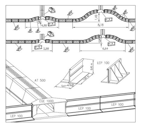
The standard straight section units give 1m of installed length, whilst the curved and cambered elements that accommodate curves and gradient changes give an installed length of 0.5m. Utilising all these components enables installation across most surfaces and terrains.
